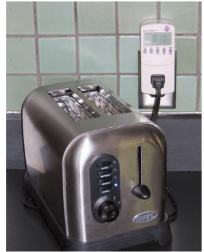
Point-of-use energy monitor.
